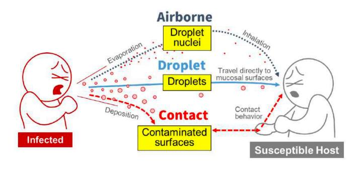
For the Airborne Transmission Mode: Where particles will typically have dimensions less than 10  $\mu$ m, decreasing the concentration of these particles can be achieved by diluting them with fresh air provided by the ventilation process
