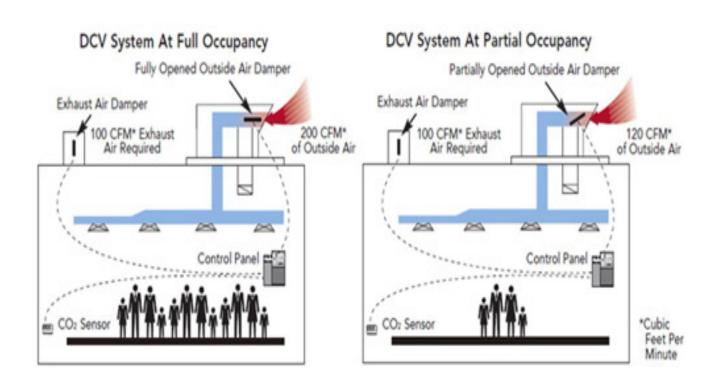
Instead of increasing the ventilation and fresh air to the maximum to remove the airborne. Like DCV that is based on CO2, we can optimize DCV based on PM by adding PM sensors in the zones.
